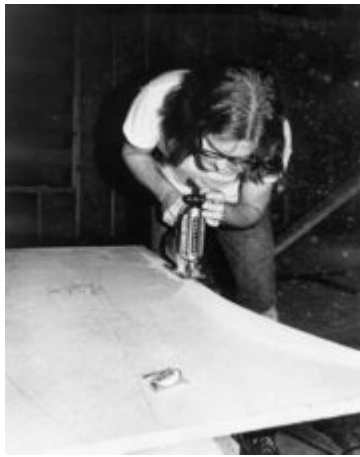
Engineer (Joe Sheets) cutting polycylinder forms. Alpha Audio Studios photo.
