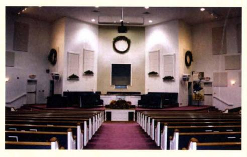
double STC or absorption. Doubling absorption thickness won't halve the room's reverberation time (RT60). To halve the reverberation time of a room will require one quantity of material. Bringing the reverb time down to one-quarter will require the same amount again. It is not linear but rather a geo-
